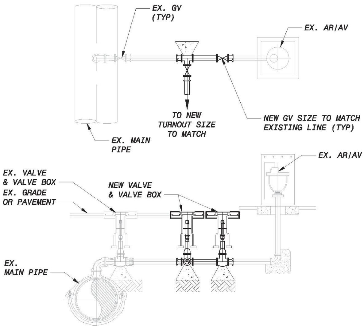
Fig. 3-5: Typical Branch Line from Air Valve Connection
