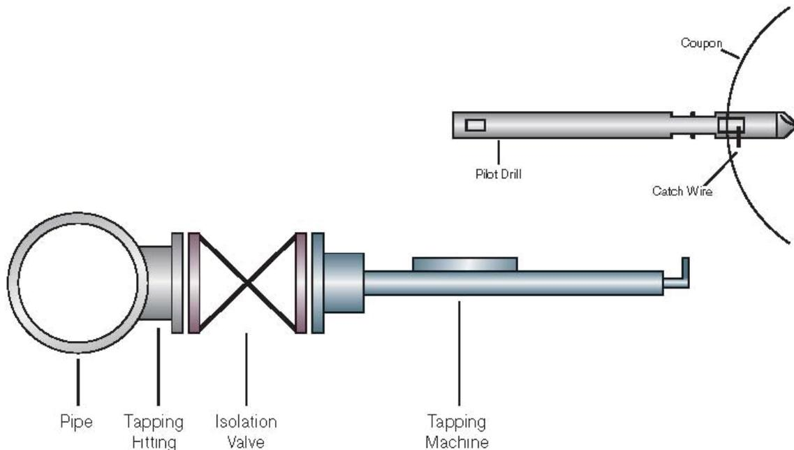
**Fig. 3-2 - Typical Hot Tapping Assembly**
