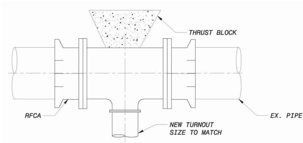
**Fig. 3-3 - Typical Cut-In Tee**
