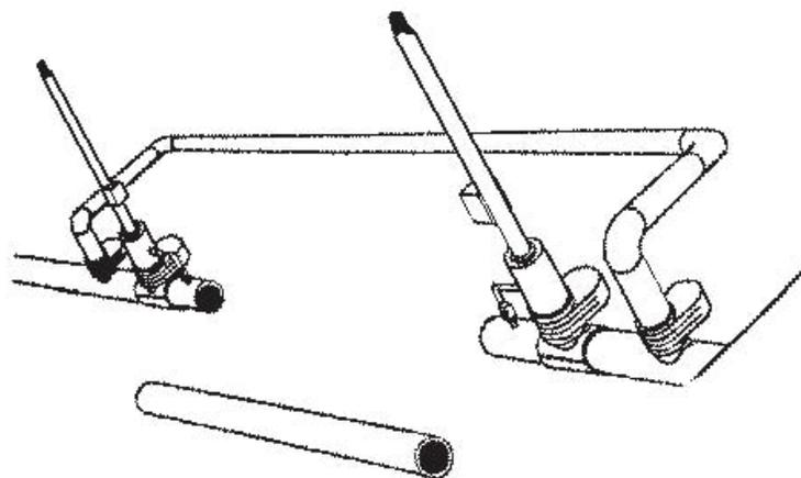
**Fig. 3-1 - Typical Bypass System Using Hot Tap**
