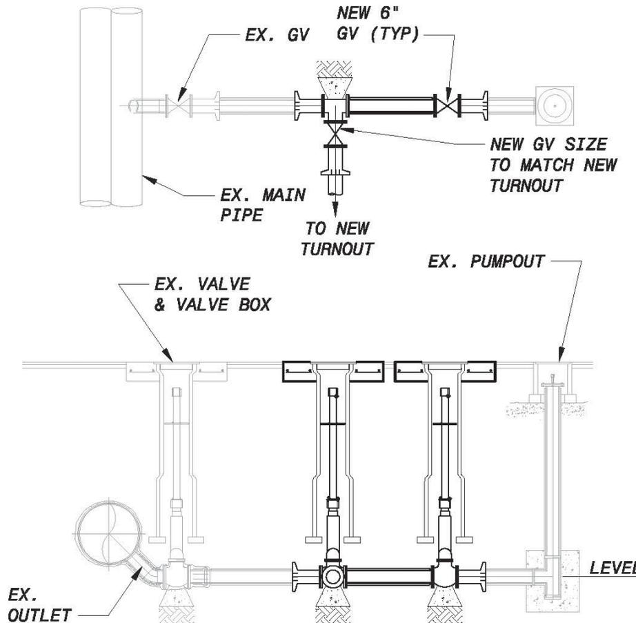
**Fig. 3-4 - Typical Branch Line from Pumpout**
