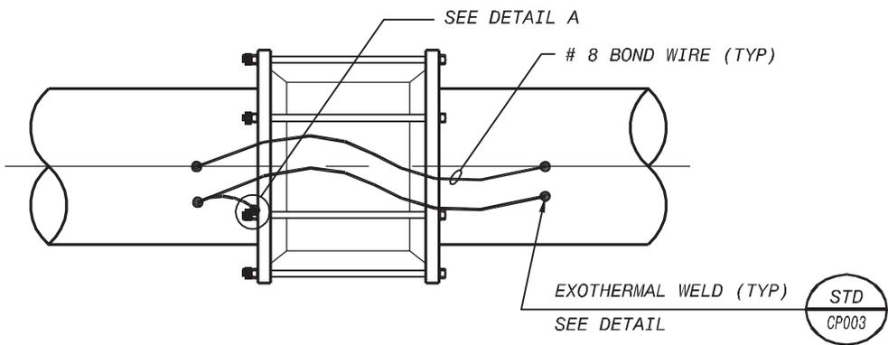
**FLEXIBLE COUPLING PIPE JOINT**
