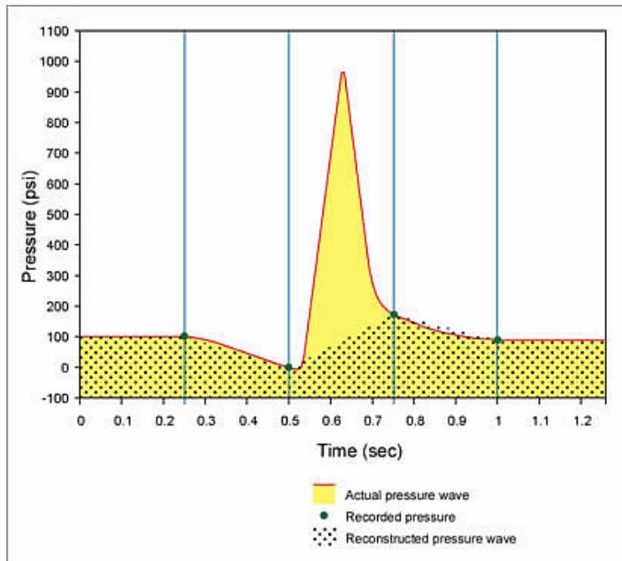
Figure 2 - Digital data collection with insufficient sample rate
