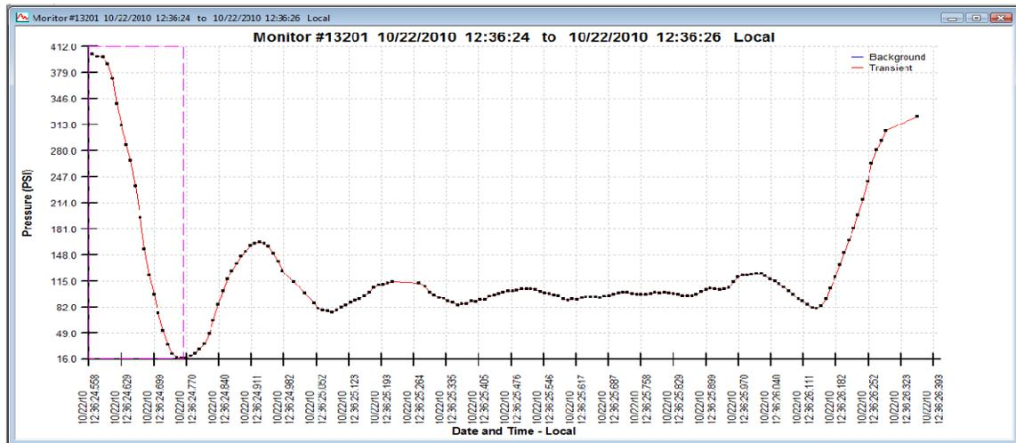
Figure 9 – TP-1 Graphical Results for Pipeline Rupture on 22 Oct 2010 at Stenner Creek
