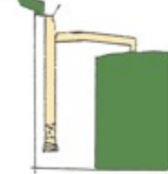
The simplest first flush system is a closed pipe before the intake. Once it fills the water goes into the tank. Annual maintenance consists of seasonally unscrewing the cap at the bottom of the pipe to flush out debris.
