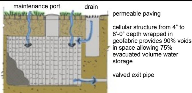
Allows paved area to also be a water retention area.
