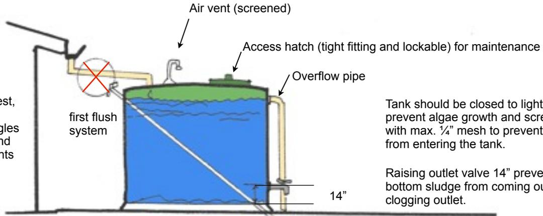
Tank should be closed to light to prevent algae growth and screened with max. 1/4" mesh to prevent pests from entering the tank.
