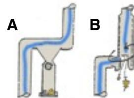
With the increasing popularity of cisterns, first flush accessories are now being produced. (A) A ball valve float seals off the first flush water and debris. (B) A screen and pipe cleverly designed to use centripetal force to swirl the water in such a way that debris drops out which also eliminates maintenance on the first flush system.
