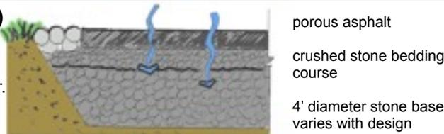
Less expensive than PICP or PCP, initially can release hydrocarbons into runoff.
