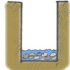
3. Put about 2" of gravel in the bottom of each hole and pre-soak holes overnight.
