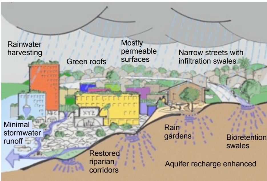
The basic LID strategy for handling runoff is to reduce the volume and decentralize flows. This is usually best accomplished by creating a series of smaller retention and detention areas that allow localized infiltration instead of carrying stormwater runoff to remote collection areas to be treated. This is accomplished by specific LID techniques, shown in recipe cards A-H, to perform the LID functions listed above.
