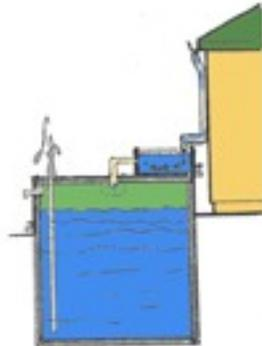
First flush can occur on a below grade tank with a small debris tank as shown here.
