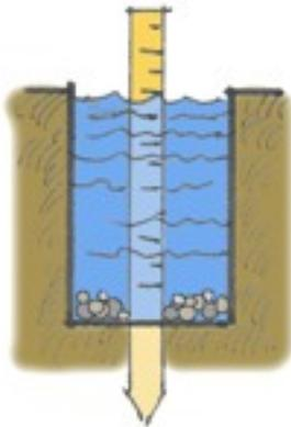
4. Pour water into the holes at least 8"-10" above the gravel. Using a stake marked at 1/4" intervals, measure water level drop at 30 minute intervals. Refill after each measurement.
