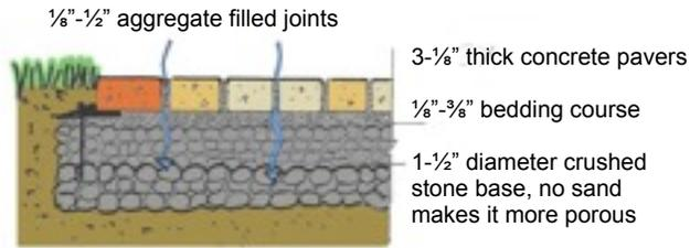
Highest loading capacity, aggregate in joints interlock units and help transfer loads.
