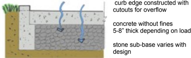
Both pervious concrete and paving asphalt have slower water passage rates and may require thicker bases for water storage.
