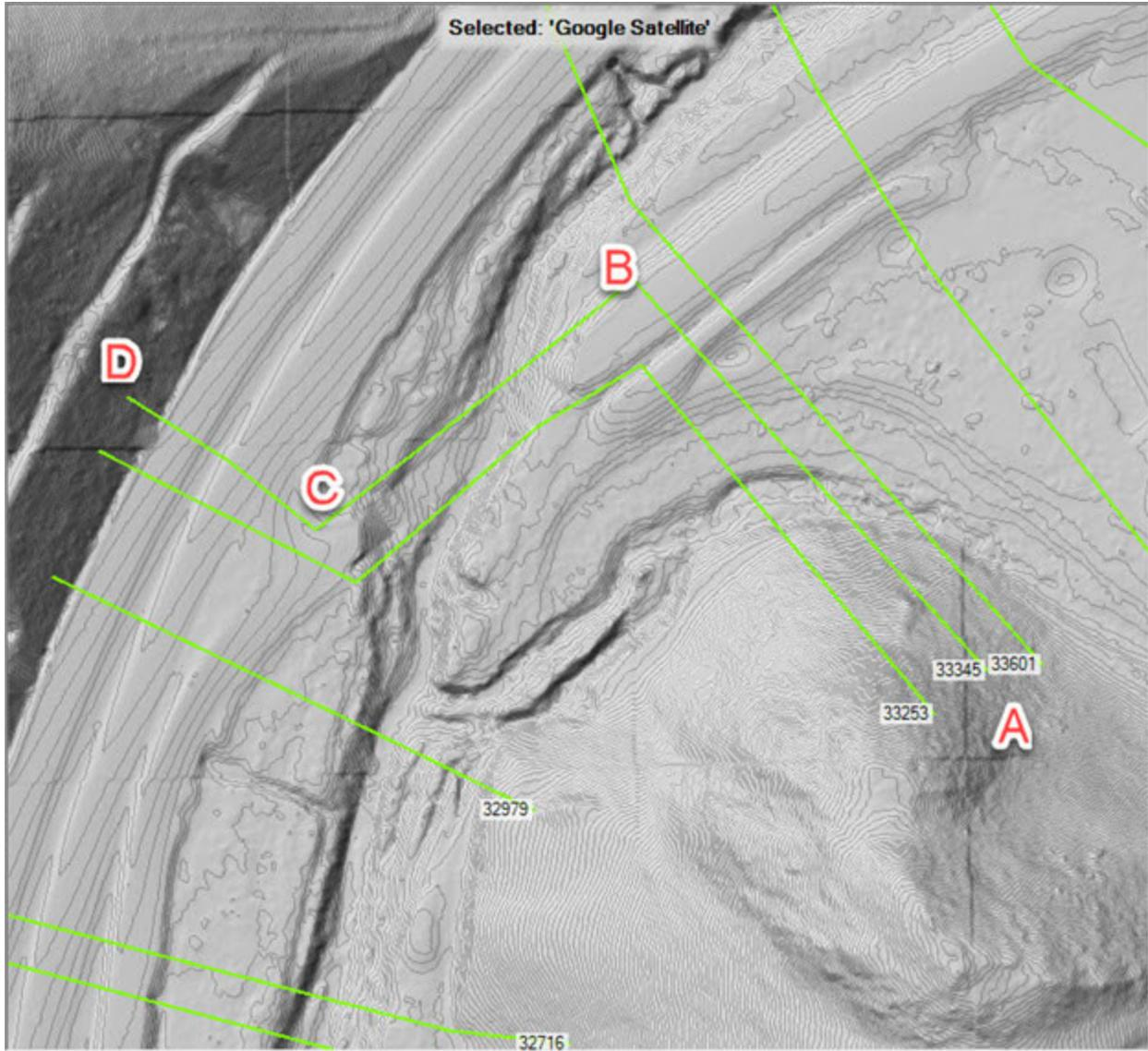
Figure 5. Higuera Street Bridge with terrain and FEMA model cross sections
