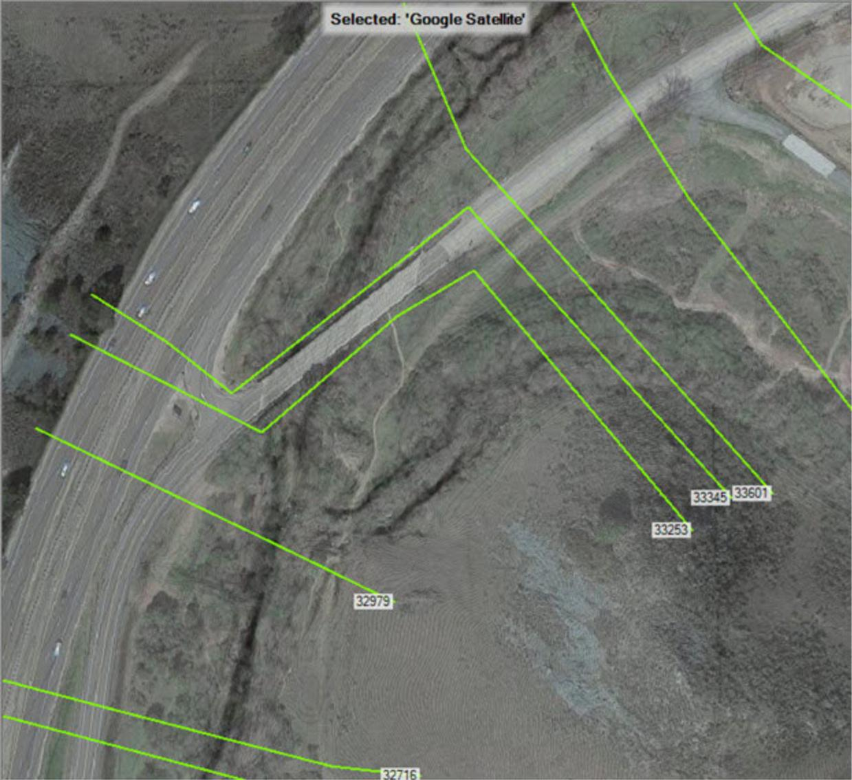
Figure 4. Higuera Street Bridge with FEMA model cross sections
