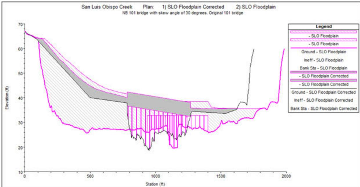
Figure 2. Comparison of the FEMA geometry (cross hatched) to the changed geometry (shaded gray) of the upstream face of the northbound Highway 101 bridge.
