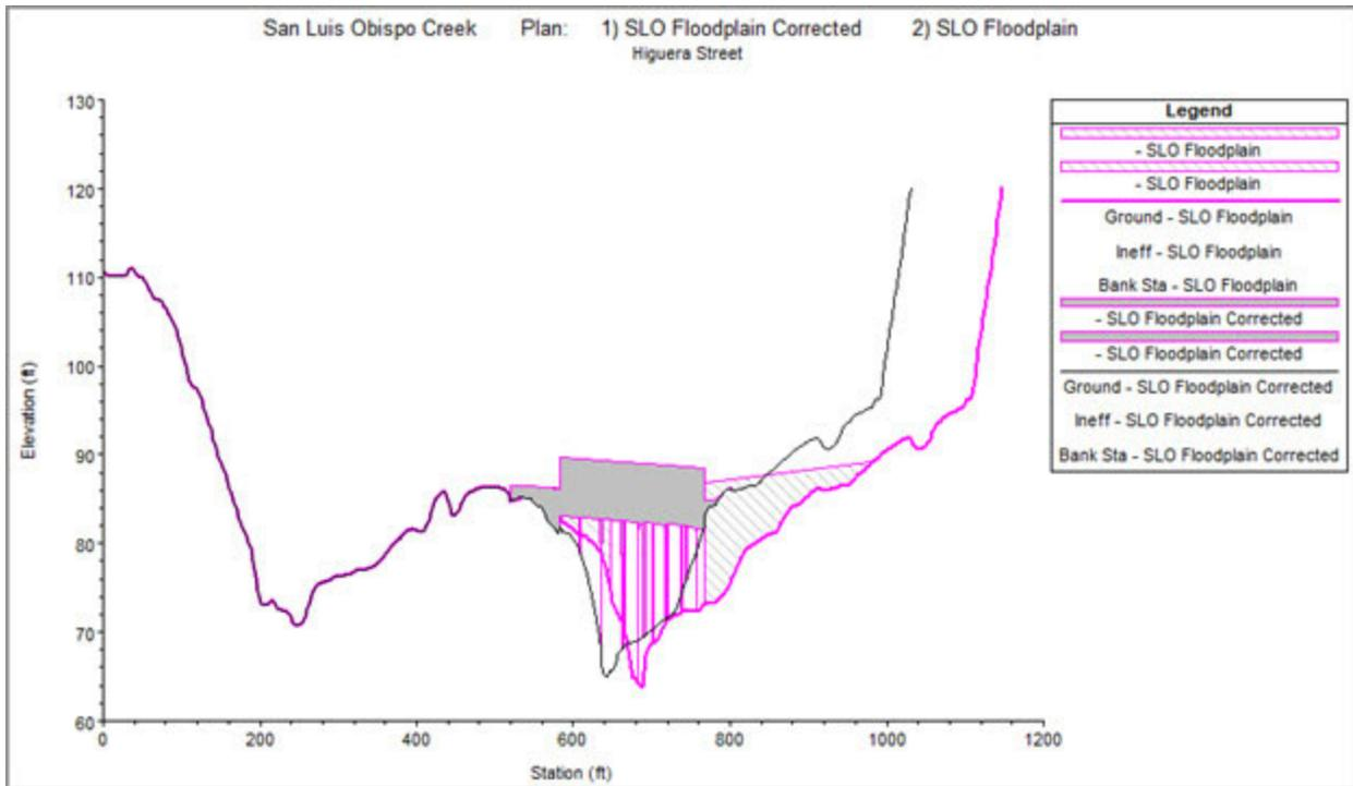
Figure 8. Comparison of the FEMA geometry to the changed geometry for the Higuera Street Bridge (RS 33278)
