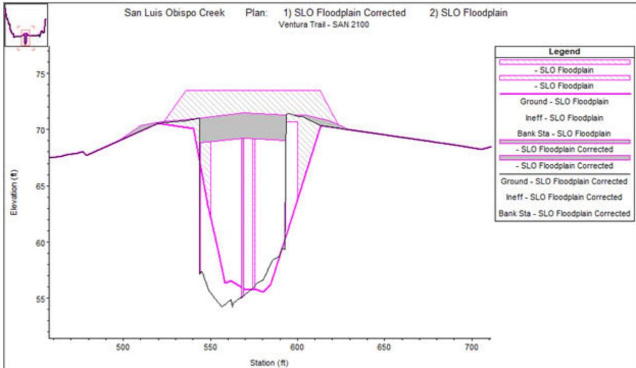
Figure 3. Comparison of the FEMA geometry (cross hatched) to the changed geometry (shaded gray) for the Bunnell Bridge (RS 29399)
