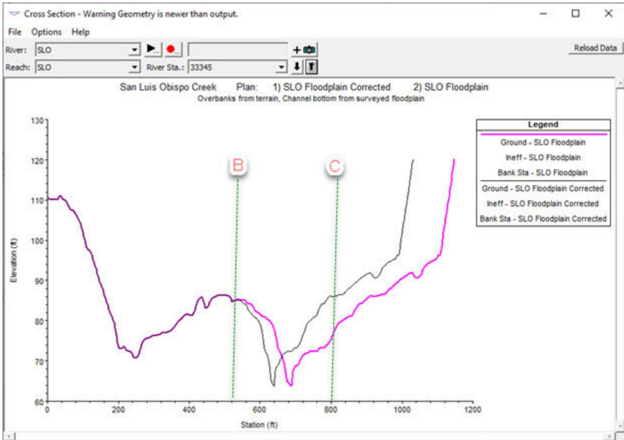
Figure 6. Comparison of RS 33345 cross section data between FEMA (magenta) and changed (black) with segment between B-C skewed 45 degrees
