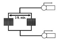
26. Split suctions must be plumbed so they are hydraulically balanced. See diagram below.
