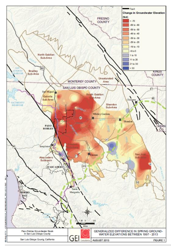
Figure 4.1 Generalized Difference in Spring Groundwater Elevations between 1997-2013
