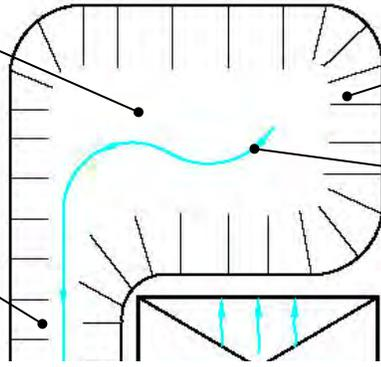
Sides should be at 3:1 minimum slope
