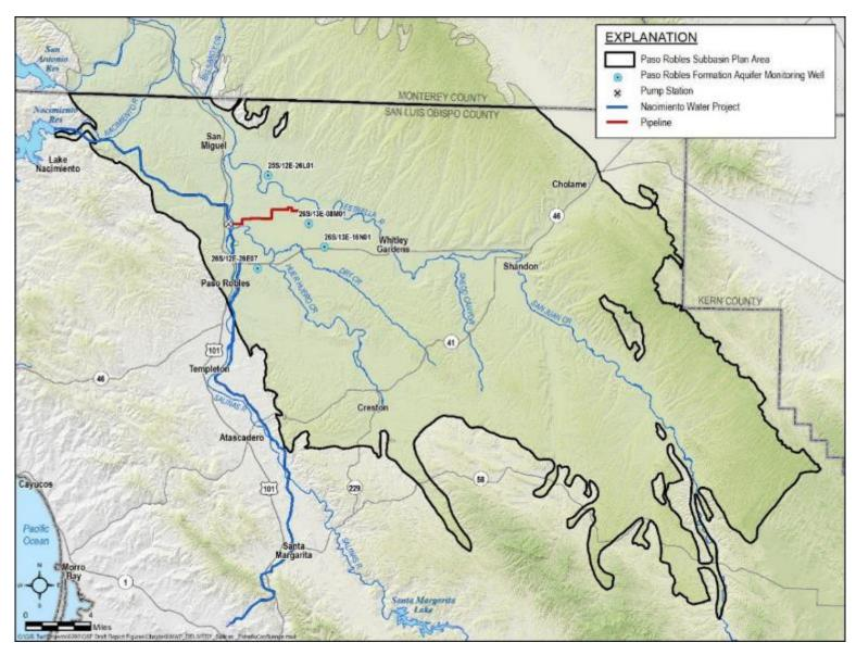
Figure 9-9. Conceptual NWP Delivery North of City of Paso Robles Project Layout
