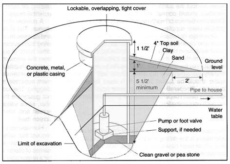
**Figure 6.** In the shoreline cistern, a 24- to 36-inch diameter cistern is dug down into the *low water* water table. A plastic, concrete, or metal liner prevents caving in and serves as a holding area for water infiltrating from the water table.
