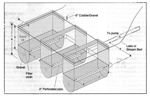
The time period between backwashes will depend upon the amount of water drawn through the filter on a daily basis and the amount of particulate matter in the water. If the homeowner's pump is not sufficiently powerful to accomplish this, it may be necessary for a plumbing contractor to perform the operation utilizing a more powerful portable pump. If a gallery cannot be backwashed, it may be necessary for the filter sand to be manually "fluffed up" or replenished by a diver.
