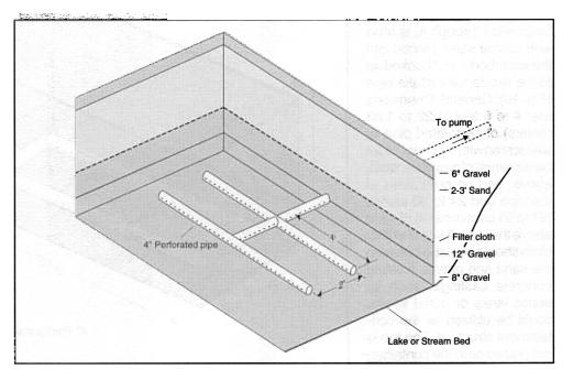
**Figure 9.** In a raised fill sand filter, perforated pipes or well screen are laid upon a layer of gravel placed on the river/lake bed. The pipes are covered with a raised fill of gravel and sand which is then covered with gravel and crushed stone or cobble.
