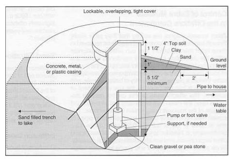
**Figure 7.** Where hardpan or bedrock near the surface precludes water infiltration into a shoreline cistern, a sand-and-gravel-filled channel can be installed between the cistern and the water source.
