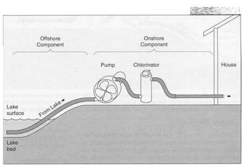
Figure 5. An in-line chlorine injection system, dosing at 0.25 ppm TRC every time the pump operates is designed to prevent the settling and growth of zebra mussels; it does not keep out shells.
