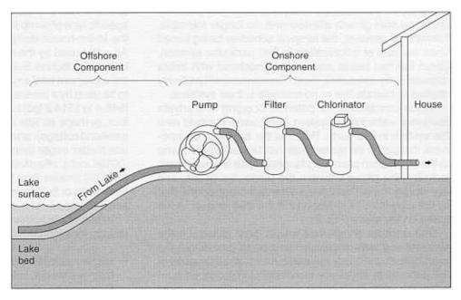
**Figure 5a**. The combination of a 25–50 micron (absolute) in-line filter capable of filtering (250–400 gpd for a year-round home of a family of four) installed in combination with an in-line chlorine injection system, dosing at 0.25 ppm TRC whenever the pump runs, should ensure that the onshore component will remain mussel-free and will improve the quality of the water in the process.
