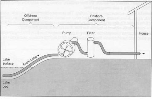
**Figure 4.** A 25–50 micron (absolute) in-line filter capable of filtering the total water consumption needs of a household (250–400 gpd for a year-round home of a family of four) installed in the onshore component to keep zebra mussel veligers and shells out of a house's interior plumbing.
