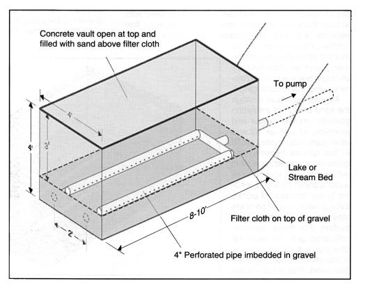
**Figure 10.** An enclosed or prefabricated sand filter constructed of a perforated pipe running lengthwise through a concrete, steel, or plastic box filled with coarse sand and placed into a waterbody is a lower cost alternative suitable for seasonal or weekend cottages.
