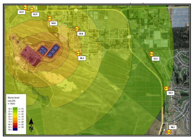
Figure 4.12-3 Modeled Noise Level Contours: Leq
