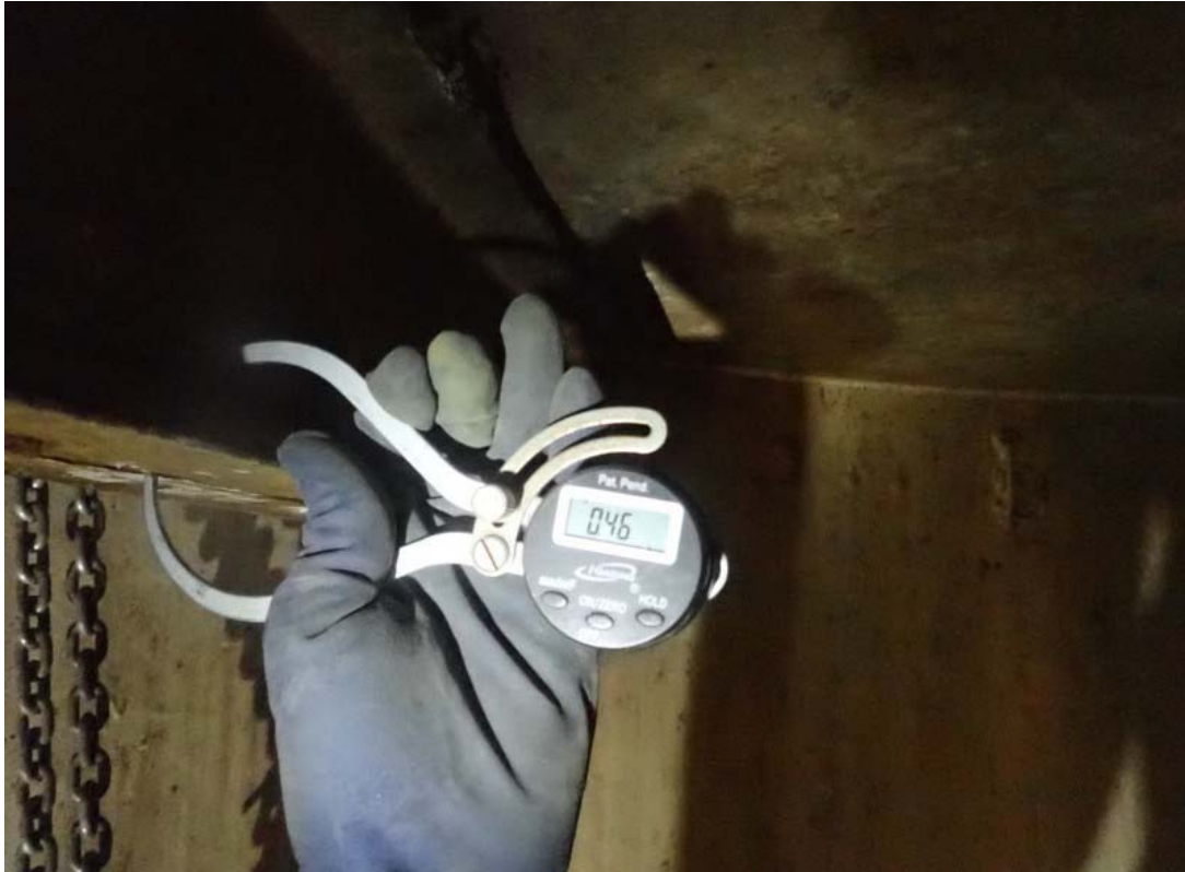
Calipers were used to measure flange thickness in the sample areas where corrosion was estimated to be the worst.
