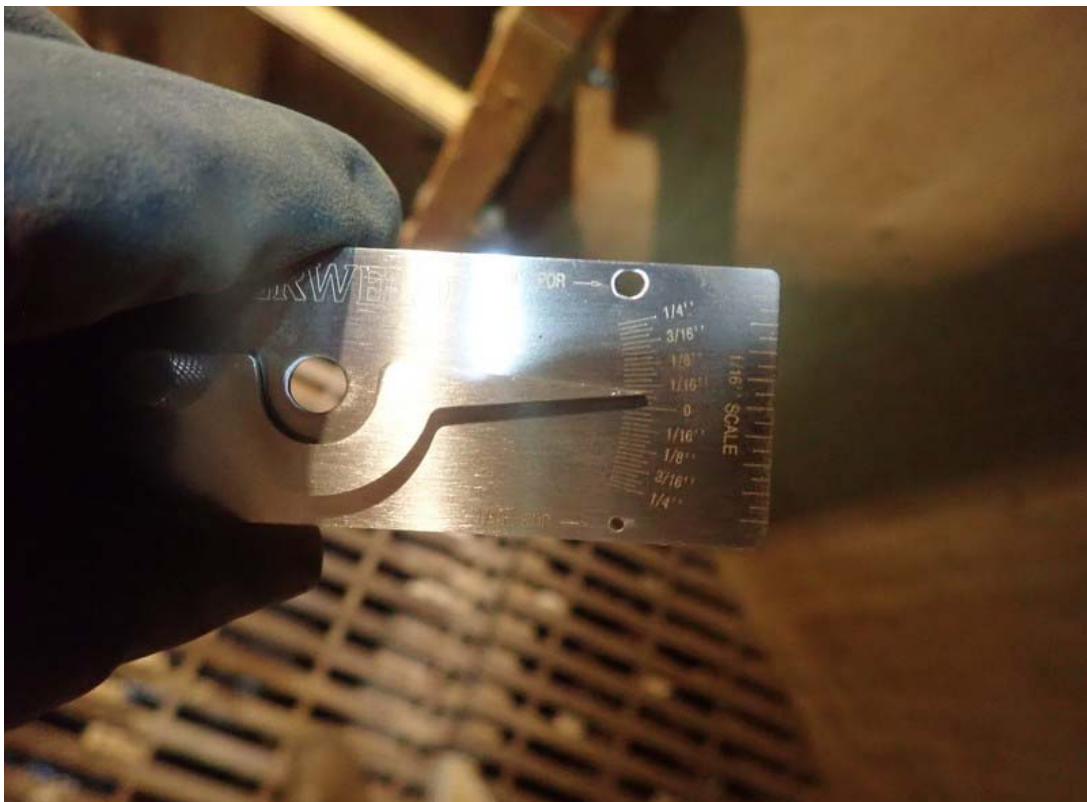
Material loss was measured as 3/64" in the worst area of localized corrosion on the hoist beam web.
